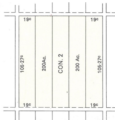
Figure 3: The single front survey system, used from 1783 to 1818. As depicted here, each lot is 200 acres (Ac.), created from surveying 19 chains by 105.27 chains (1 chain = 66 feet/ 20.12 metres) (Gentilcore 1969:61)
