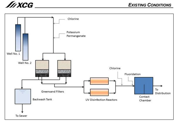
Figure 8 Prospect Park Process Flow Diagram
