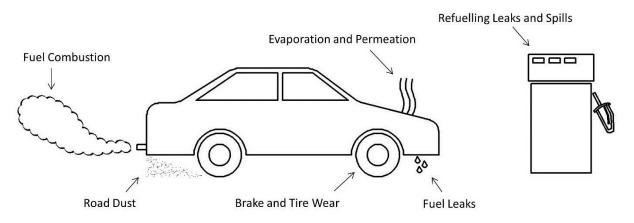
Figure 2: Motor Vehicle Emission Sources
