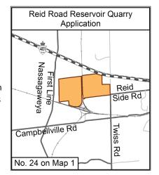
Based on the application notification documents, JDCL is proposing approximately 29.4 ha for licencing, with approximately 25.7 ha proposed for extraction. The applicant estimates sand and gravel reserves at approximately 500,000 tonnes and dolostone at about 12.5 million tonnes. As per the application's Site Plan and Summary Statement Report (June 2018), the maximum annual tonnage is proposed to be 990,000 tonnes.
