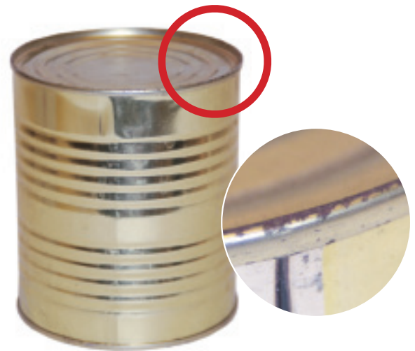
Pitted rust or leaking
