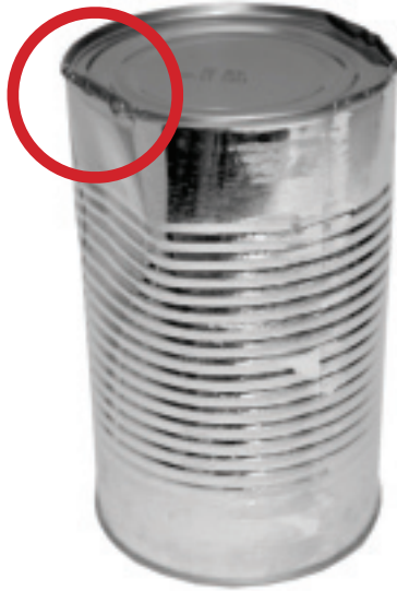
Dented at junction of side and end
