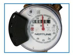
For the meter below, shine a bright light on the solar strip to display numbers.
