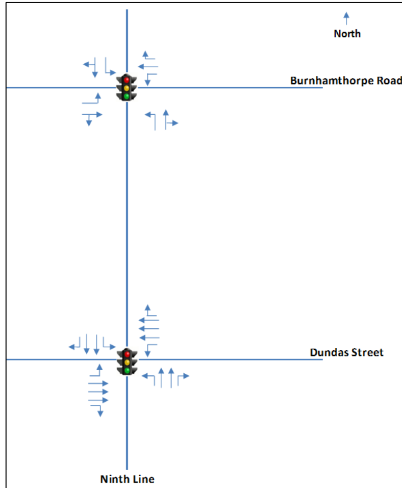
Figure 2: Existing Lane Configuration
