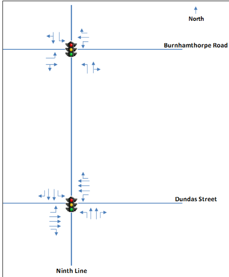
Figure 4: Existing Lane Configuration (2015)
