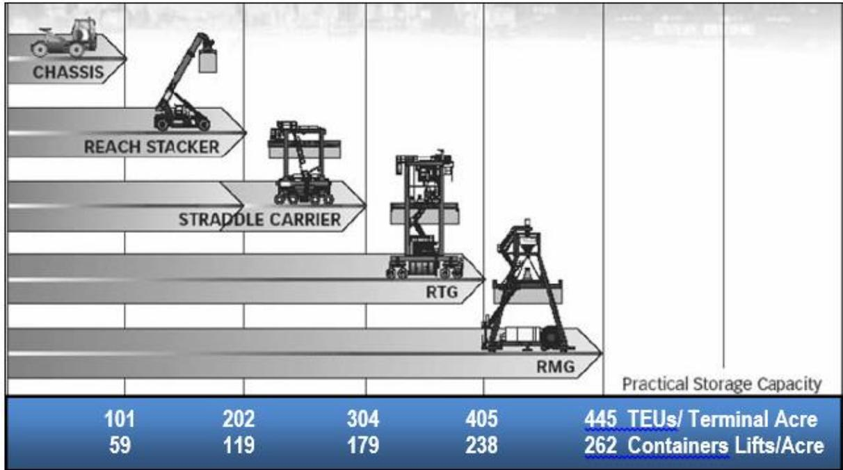
Considering the potential productivity benefits of the above chart, changing from a Reach Stacker yard crane system to a RTG or Rail Mounted Gantry (“RMG”) yard crane system could effectively double the intermodal rail terminal practical storage and throughput capacity.
