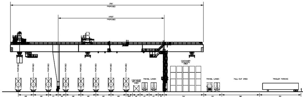
These WSC or RMG/RMC yard crane installations have proven to strikingly reduce air emissions and provide for almost silent terminal crane operations. From an intermodal rail systems standpoint, the WSC/RMG/RMC can dramatically increase terminal throughput and network connections for the railroad while improving facility safety and all while operating in a semi-automated or fully automated operational mode.
