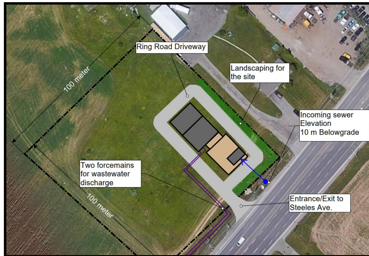
Shown above: preferred wastewater pumping station site layout
