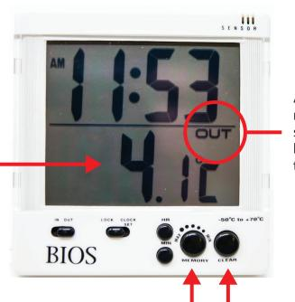
Always make sure the screen reads 'OUT'. If it reads 'IN', slide the in/out button on the bottom left hand corner of the thermometer.
