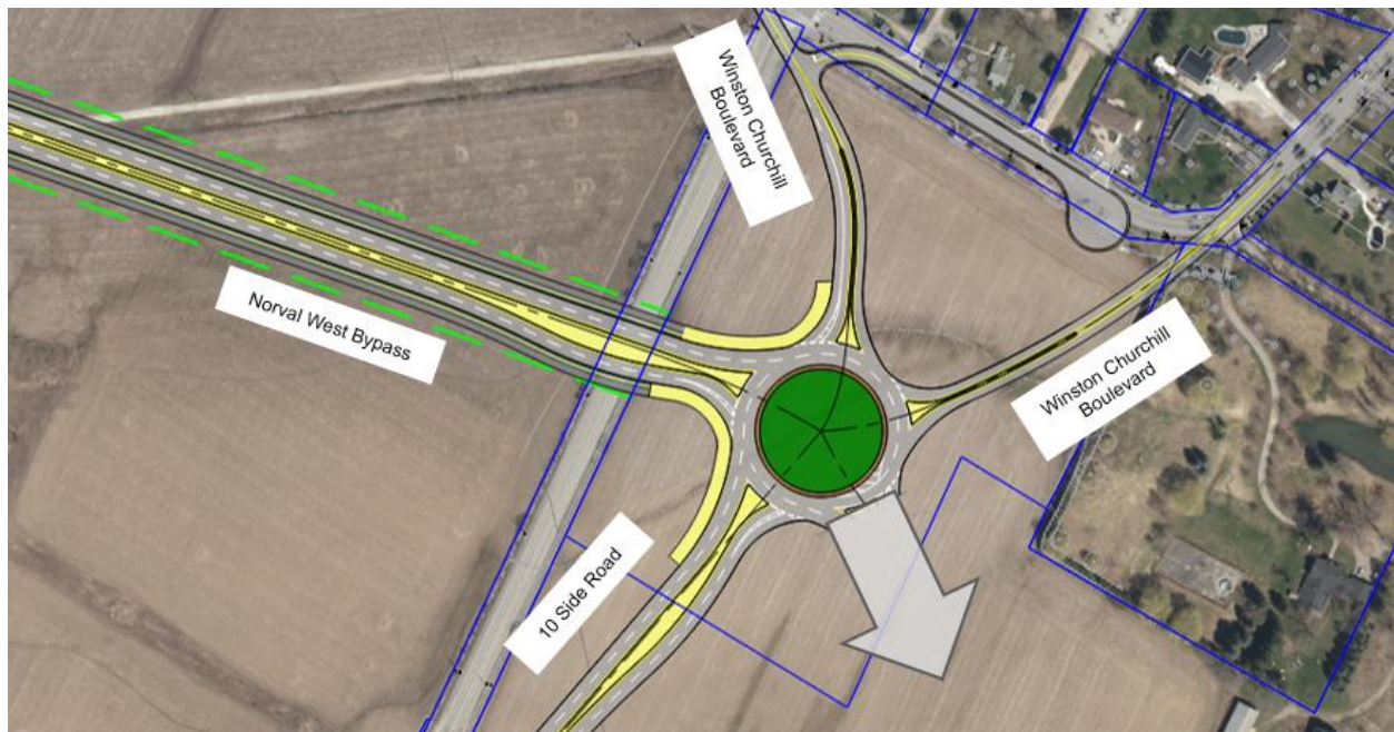
Figure 23: 10 Side Road Intersection Alternative 2
