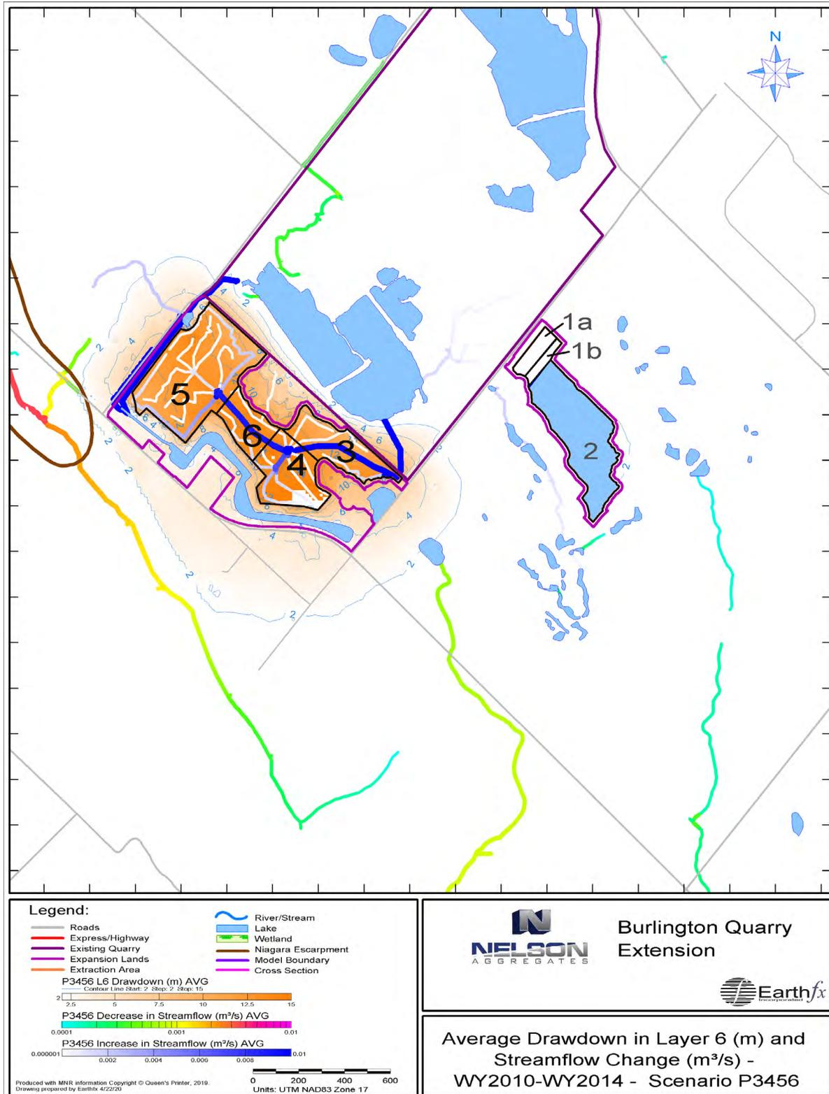
Figure 2: Average simulated drawdown in Model Layer 6 (m) and increase/decrease in streamflow (m<sup>3</sup>/s) for WY2010 to WY2014 under Scenario P3456.
