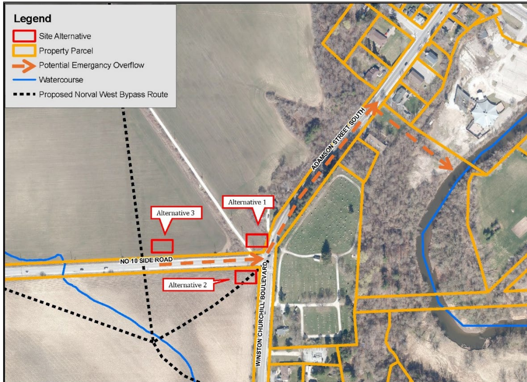
Figure 13: Potential Emergency Overflow Route
