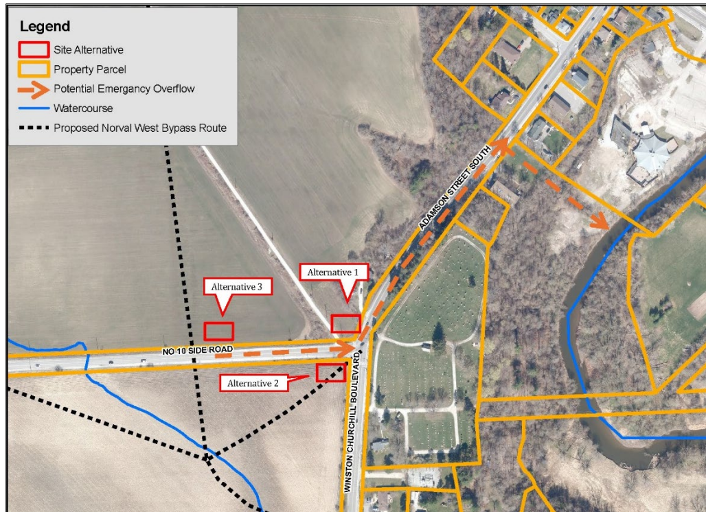
Figure 13: Potential Emergency Overflow Route.
